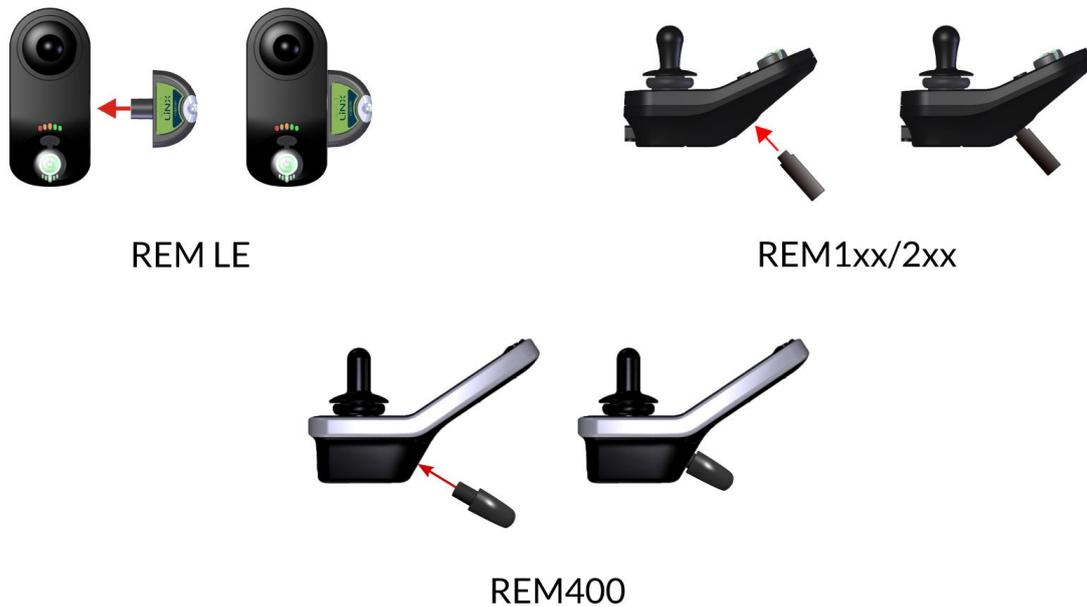
Figure 4: Inserting the LiNX Access Key
