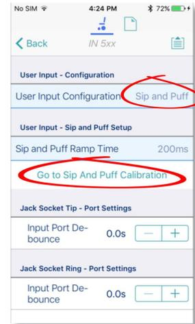
**Figure 45: Open sip and puff calibration**
